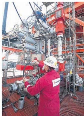
PRESSURE ON: A technician connects hydraulic hoses to Cameron's 25,000 psi DR-20 drilling chokes.
