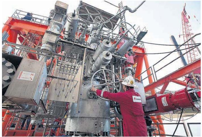
**TOUGH KIT:** Cameron says its 25,000 psi, fully cladded surface production tree is the first-to-market system for ultra-high pressure, high-temperature applications.
