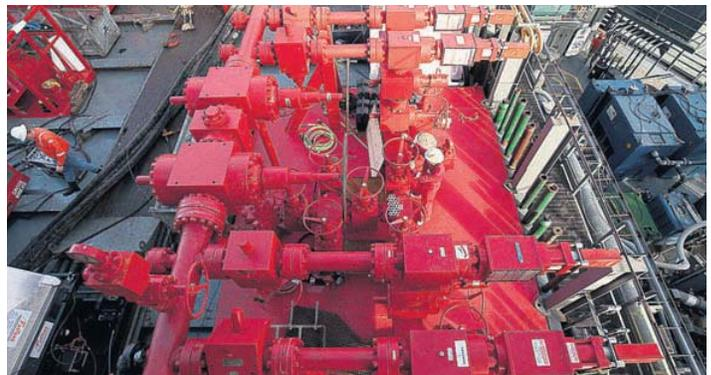
**DESIGNED AND QUALIFIED:** Cameron's 25,000 psi partially cladded drilling manifold was transported on a complete skid to the offshore platform.
