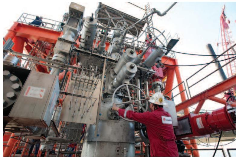
**For the 25,000-psi production tree, the valve and choke, both critical components, and the tooling required for installation did not exist. (Source: Cameron)**
