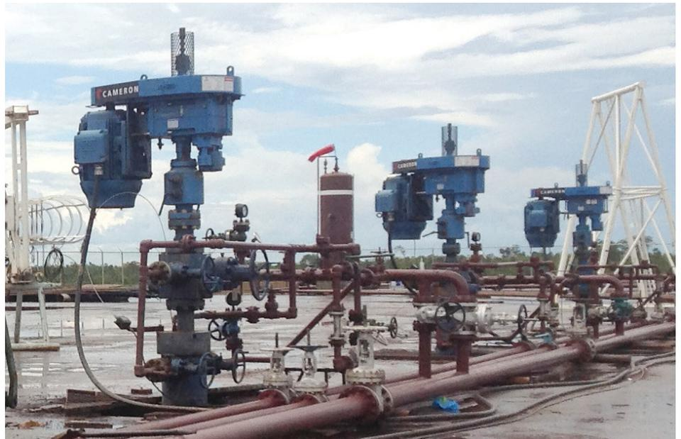
*PetroMiranda used the FC fast connect HT wellhead system—custom engineered for heavy oil operations—on all its heavy oil wells in Venezuela because of the system's ability to withstand corrosive environments and temperatures up to 650 degF, reduce installation time, and eliminate the need for expansion joints.*
