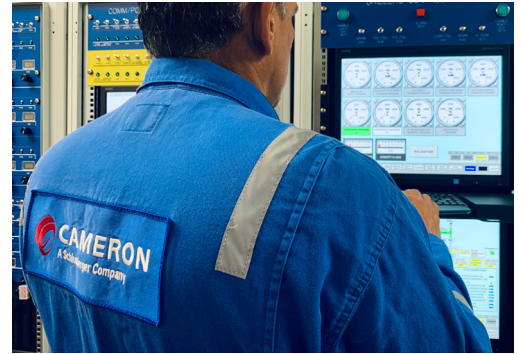
Cybersecurity-enabled Cameron BOP control system simulator.
