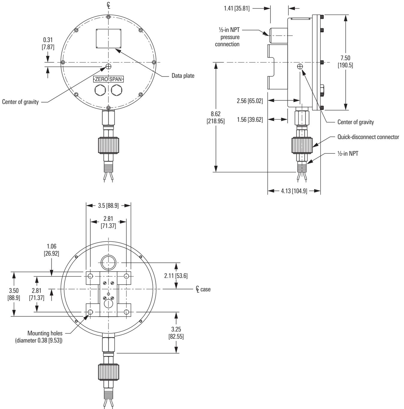
BARTON 763A transmitter dimensions, in [mm].
