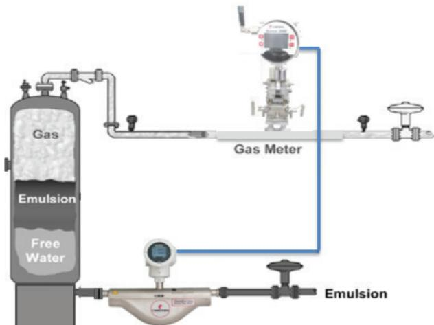
*Two-phase separator using a Coriolis flow meter for watercut measurement.*
