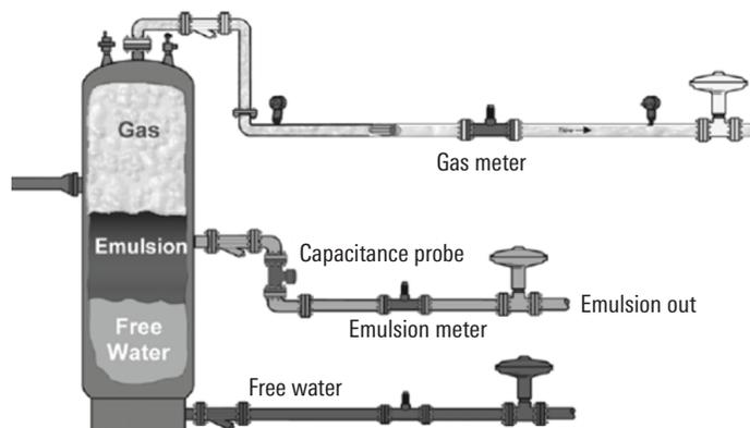
*Three-phase separator using a water and oil ratio analyzer (emulsion meter) for water-cut measurement.*
