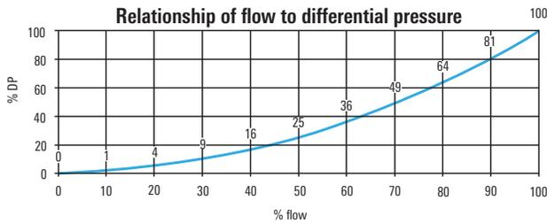
What is usually observed is that turndown is not caused by the limitation of the differential-pressure-producing device but by the ability to precisely sense the differential pressure. DP sensor stacking is a method to reduce uncertainty. In regard to the values presented in the subsequent example, the evaluator should consider possible limits and the additional uncertainty of the specific DP producer.
