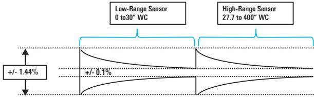
The Cameron Scanner 3100 flow computer offers triple sensor-stacking capabilities to support further reduced uncertainties or higher turndown capabilities.
