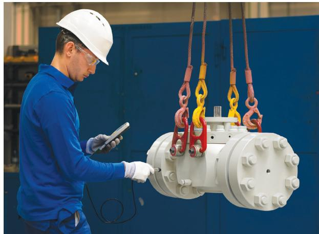
**FIGURE 1. Designed using finite-element analysis and computational fluid dynamics, the ball valve provides enhanced sealing in a compact design. (Source: Schlumberger)**
