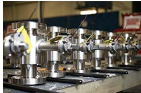
The piping connections selected for cryogenic service are usually flanged or welded configurations. Either of these connection types can handle a wide pressure range; the majority of applications being ASME Classes 150-600 (and some applications up to Classes 1500 and 2500).
