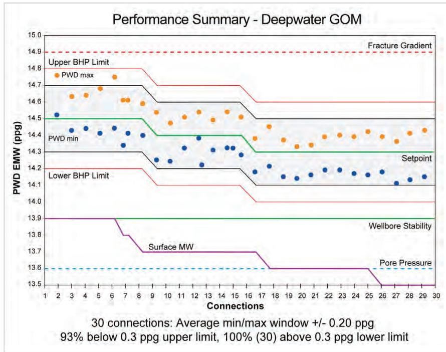
The performance summary is the record of minimum and maximum BHP that occurred during every connection managed by the system during one of the Auger wells. In this well the system managed BHP in 30 connections during which time the static MW was reduced in stages from wellbore stability to below pore pressure. The target window for the well was +/- 0.3 ppg relative to the setpoint which changed in stages along with the MW. The DAPC system achieved +/- 0.2 ppg for 93% of the connections.
