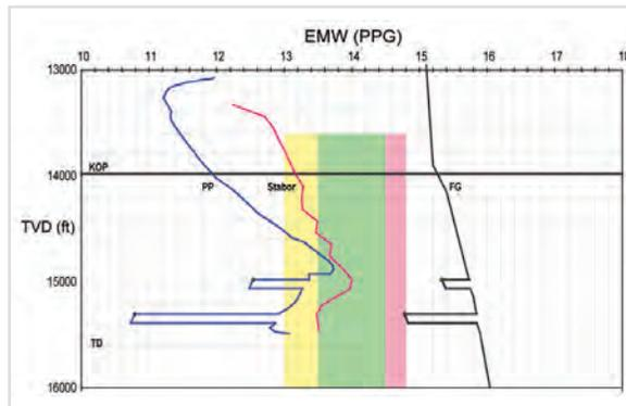
Narrow margin between fracture gradient and wellbore stability. High ECD caused by high mud weight, slim hole, and hole cleaning flow rates. Constant BHP with the DAPC system enabled Shell to reduce the mudweight and ECD, eliminate losses, and maintain stability.
