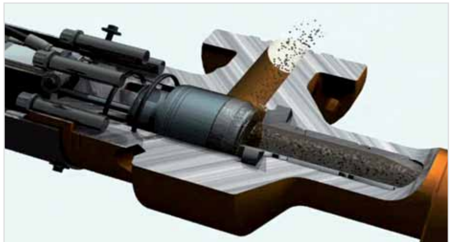
Cut-away of the AutoChoke system in operation
