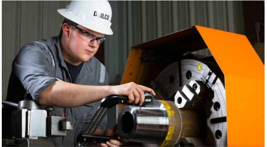
*DRILCO's tubular experts at the C-Port II facility use CNC and manual lathes to repair API, SSDS, and TSDS connections.*
